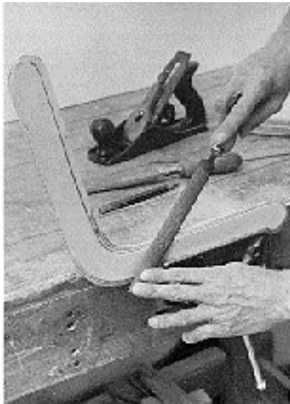
Figure 8 - 3rd position of blank. Rasp angle the same as in 1st position. The wood plane cannot be used at this or final stage of shaping Figure 9 - 4th and final position of blank. Note how the right arm is positioned behind the work at this final stage. Rasp angle as in 2nd position.
