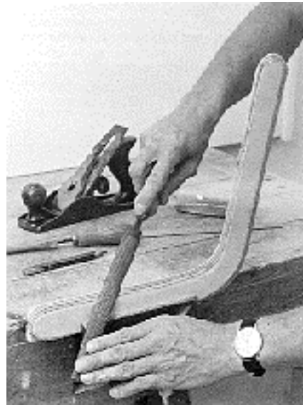
Figure 8 - 3rd position of blank. Rasp angle the same as in 1st position. The wood plane cannot be used at this or final stage of shaping Figure 9 - 4th and final position of blank. Note how the right arm is positioned behind the work at this final stage. Rasp angle as in 2nd position.
