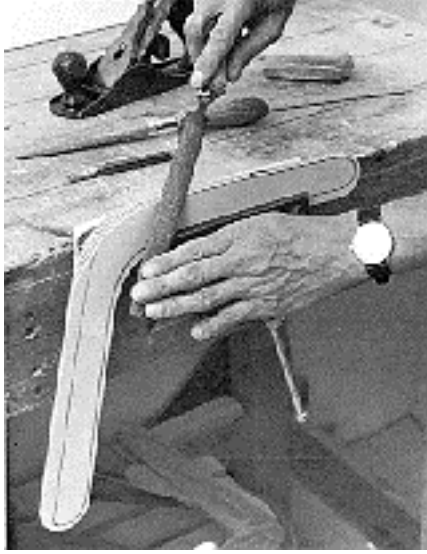
Figure 6 - 1st position of blank in the vice. Figure 7 - 2nd position of blank. Note wooden strip placed behind blank, and working angle of rasp. Here it will be necessary to hold the rasp at a slightly steeper angle to shape the trailing edge of the blade. Again the wood plane can be used at this stage, if preferred.
